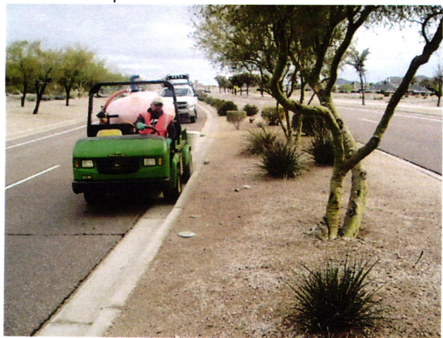
Spray rig with directional boom and traffic control
