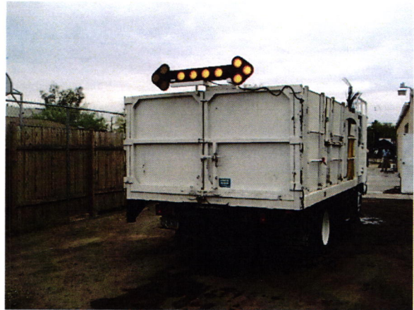
Arrow boards mounted for traffic control.
